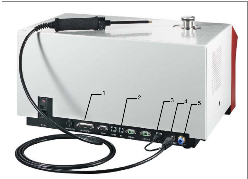
Fig. 5-2 Connections for sniffing probe
