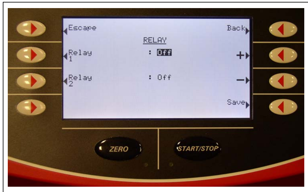
Fig. 6-36 Relay view of the "Relay" setting in the display Relay allows independent settings for the two output relays.
