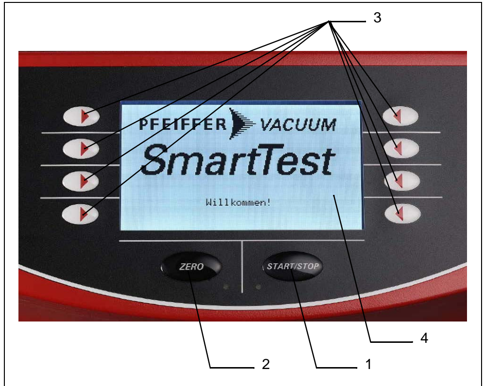
Fig. 4-1 Functions of the buttons on the display
