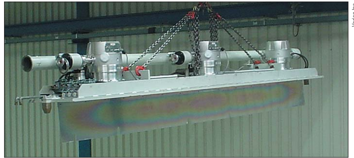
Using vacuum pumps to make architectural glass.
